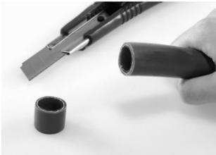
1. Using a sharp knife, cut hose end cleanly and squarely.
