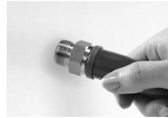
4. Hold fitting end against a flat surface. Grip hose approximately one inch from blue cap and push with a steady force until the hose bottoms inside the blue cap firmly.
