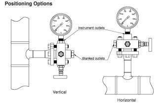
Instrument outlets can be positioned to suit horizontal or vertical process pipeline. Standard Monoflanges are supplied for horizontal installation. For vertical installation, add "V" to the valve ordering number.
